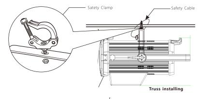
Regardless of the rigging option you choose for your PROFILE NF200RGBW-MZ, always be sure to secure your fixture with a safety cable. The fixture provides a built-in rigging point for a safety cable on the hanging bracket as illustrated above. Be sure to only use the designated rigging point for the safety cable and never secure a safety cable to a carrying handle.
